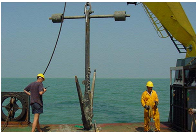
Figure 4C: Typical 1-Meter Grapnel for Recovery of Buried Cable 20
