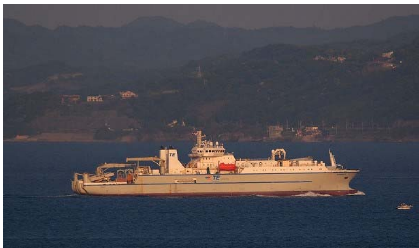
Figure 4B: A typical cable ship, the C.S. Dependable 19
