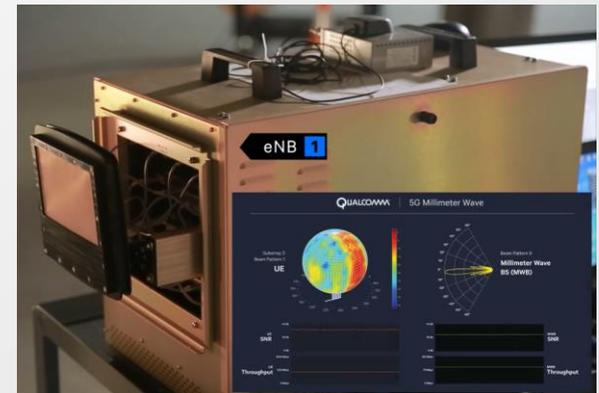
Qualcomm Research 28 GHz end-to-end prototype system demonstrates beam forming and scanning to address NLOS scenarios, improve indoor/outdoor range, and provide robust mobility
