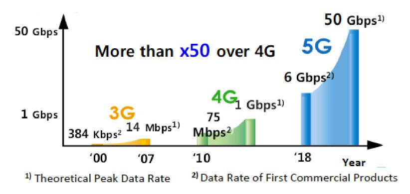
Plot of generational data rates for 3G, 4G, and 5G networks. Millimeter Wave spectrum is needed to meet 5G demand.
