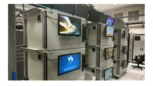
octoBox® controlled environment wireless testbed for testing real devices under controlled conditions, including interference, signal loss and multipath; ideal for interoperability, performance and coexistence testing
