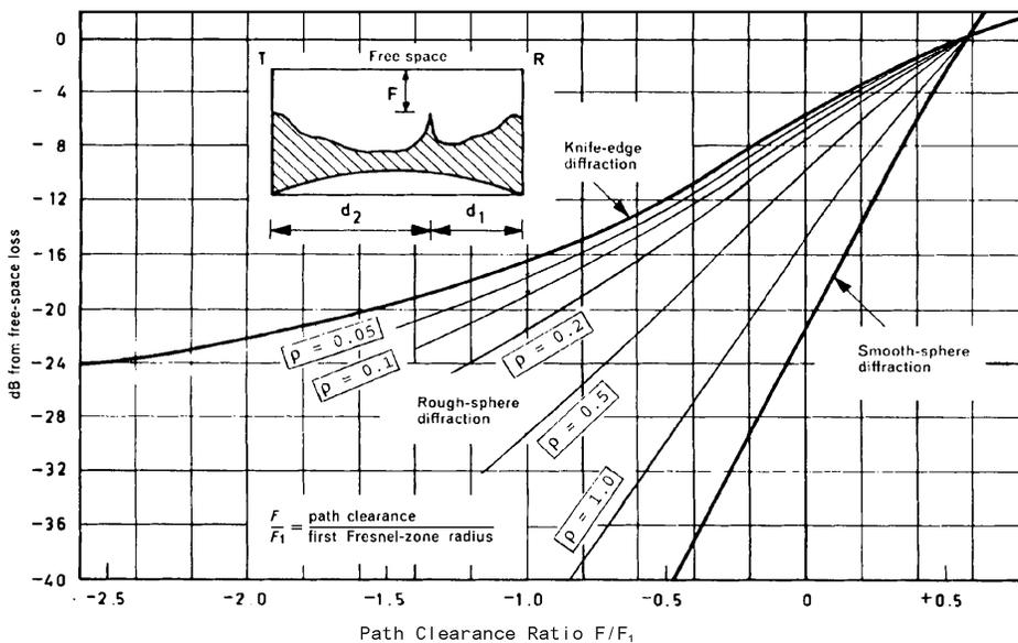
diffraction adjustments for rounded obstacles. Note: the ratio of path clearance to first Fresnel radius,  $F/F_1$  in the figure, equals the Dougherty-Maloney parameter  $\rho$  divided by the square root of 2.
